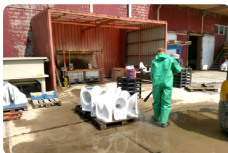
Phase 2: Pressure rinsing
