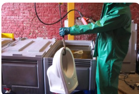
Phase 1: soaking the elements in a specific acid bath
